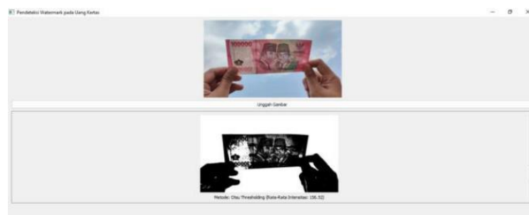
Figure 4. Segmentation result of Otsu Thresholding method
